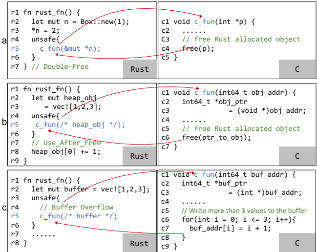
Figure 1: Sample multilingual Rust programs illustrating three kinds of memory vulnerabilities across Rust and C: a double-free in (a), a use-after-free in (b), and a buffer overflow in (c).
