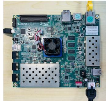
Fig. 2: Xilinx Zynq UltraScale+ MPSoC ZCU104 board
